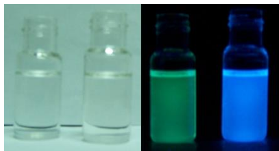
Fig. 6. The color and fluorescence changes of compound PUIO in DMSO ( 1.0 \times 10^{-4} \text{ M} ) after addition of 50 equivalents [(\text{Bu})_4\text{N}]\text{F} . Left to right: PUIO, PUIO+ [(\text{Bu})_4\text{N}]\text{F} , PUIO (emission), and PUIO+ [(\text{Bu})_4\text{N}]\text{F} (emission). Irradiation at 365 nm using a UV lamp.
